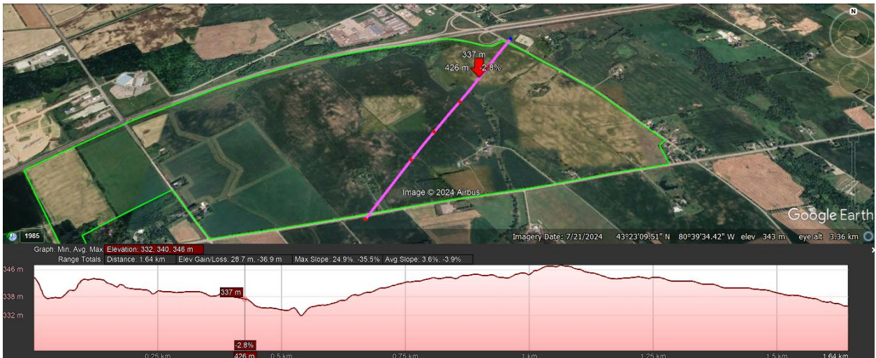
Figure 15: Elevations along the Hydro Line
