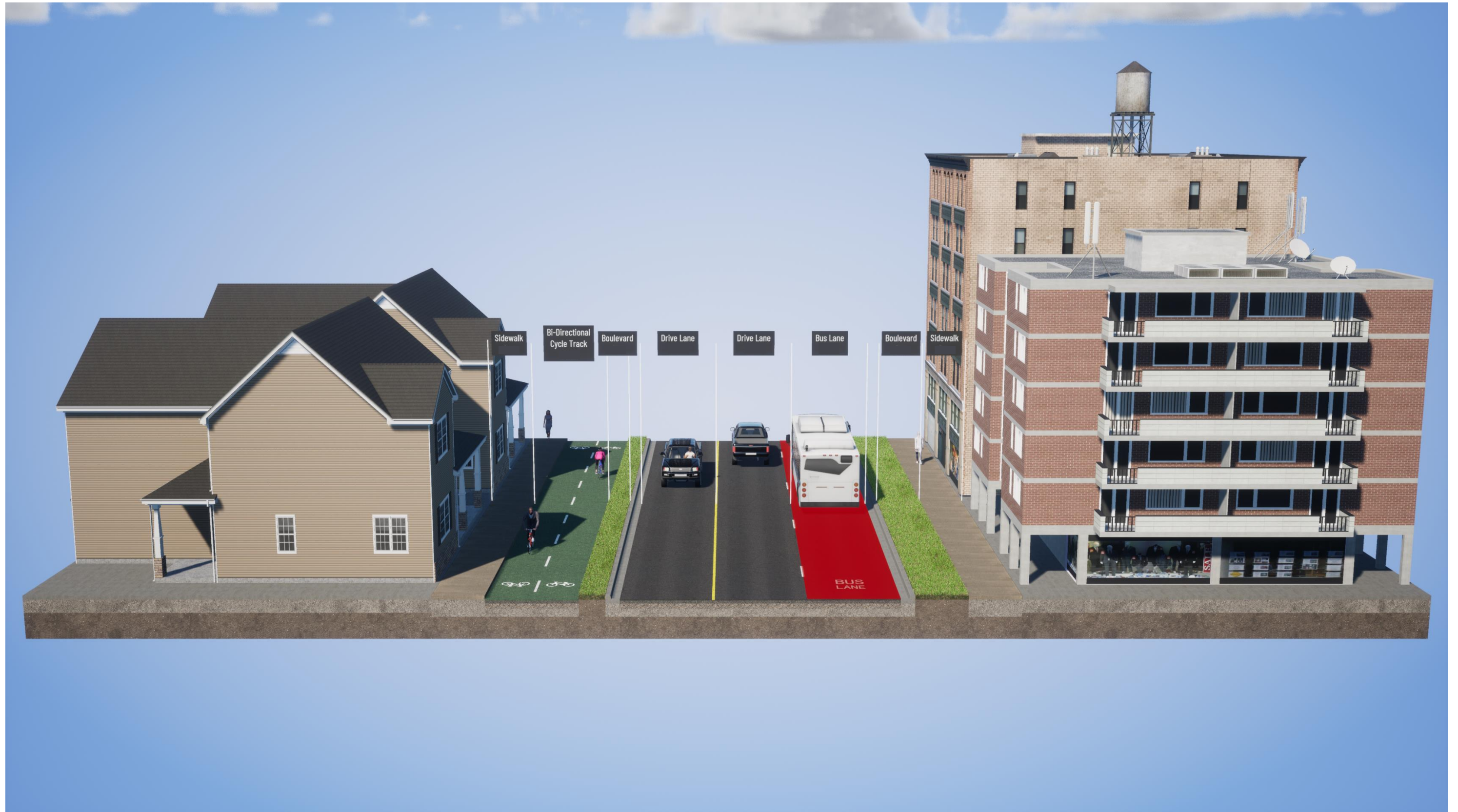
Figure 3 Proposed Victoria Street North Cross-Section in front of Rumpel Felt Co. Building (Constrained Right-of-Way)
